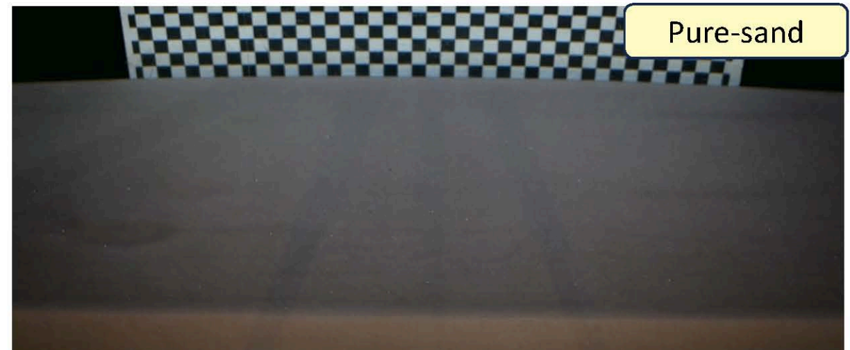
Wave ripple development in a test of pure-sand bed
