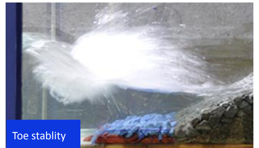
Low-crested structure with dynamic cobble beach
