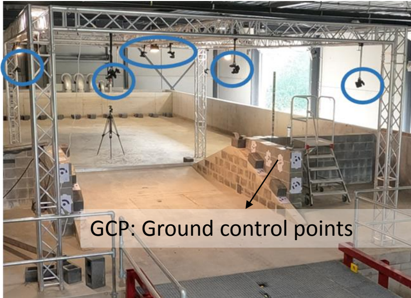
Multi-stationary synchronized cameras 10 Fixed cameras on time-lapse mode
