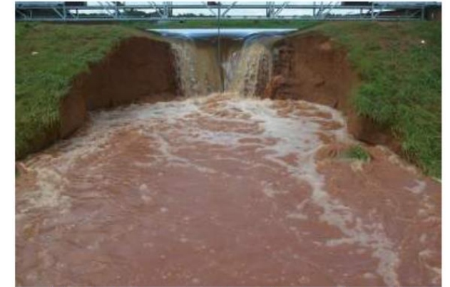
(a) Headcut erosion through a test levee [Photo: USDA-ARS-HERU Stillwater, OK. US]
