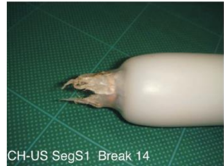
Broken cables due to the turbidity currents and submarine landslides in Kaoping Canyon subsequently two earthquakes. Hsu et al. (2008).
