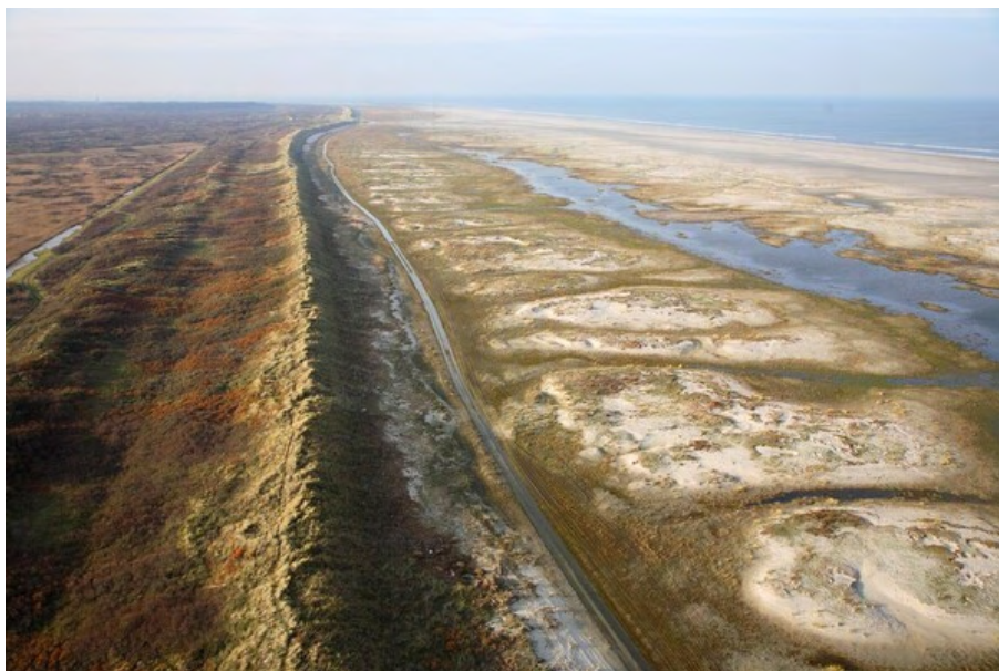
Figure 1: Aerial image of Schiermonnikoog with from left to right the salt marsh, the sand-drift-dike, the green beach, the sandy beach and the North sea (source: Beeldbank Rijkswaterstaat, Joop den Houdt).
