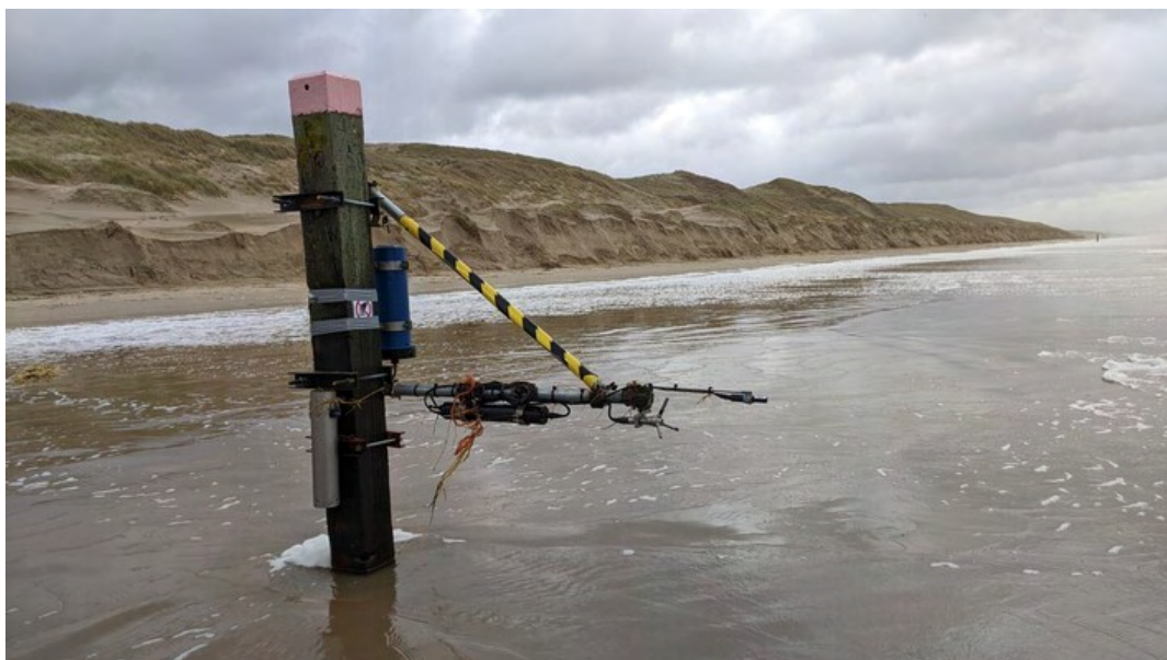
An Acoustic Doppler Velocimeter (ADV) mounted to a beach pole, with dune erosion in the background resulting from storm Pia in December 2023.
